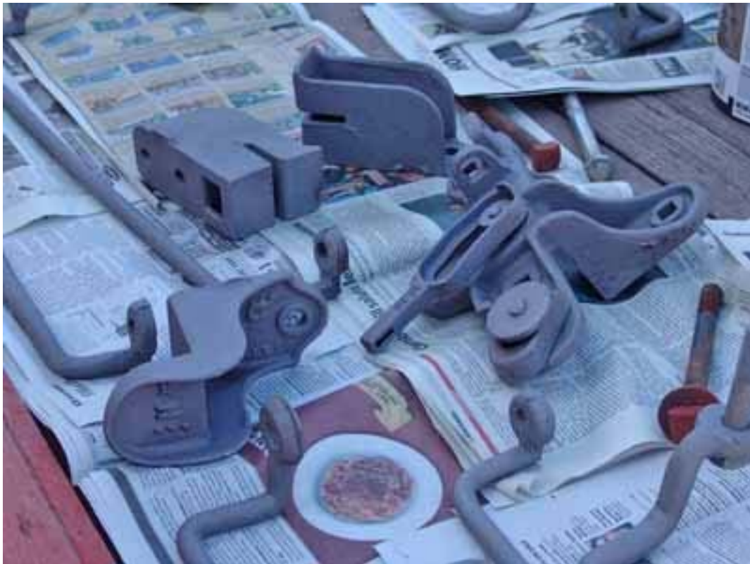
Hardware for the TC & GB box car all sand blasted and looking like new.
