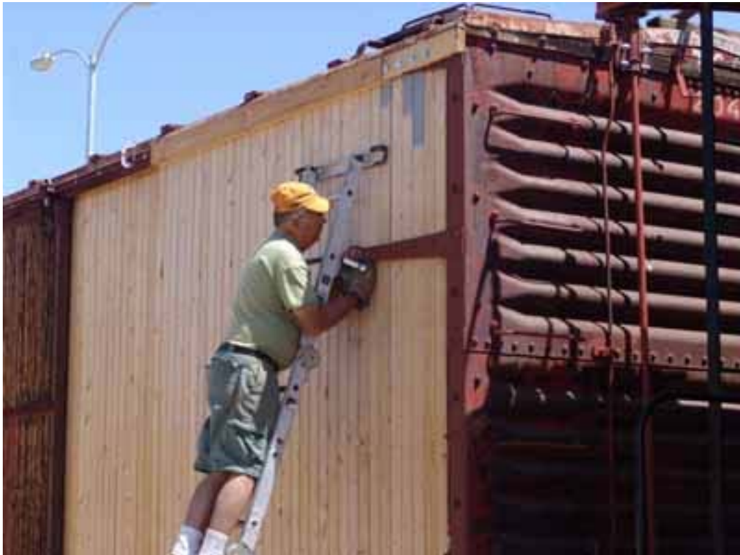
Gerry McGonigle, boy he gets around, works to get the bolt through the brace on the TC & GB boxcar.
